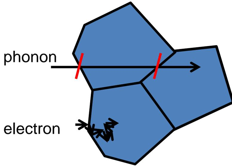
Introducing scattering centers to reduce thermal conductivity  $\kappa$
