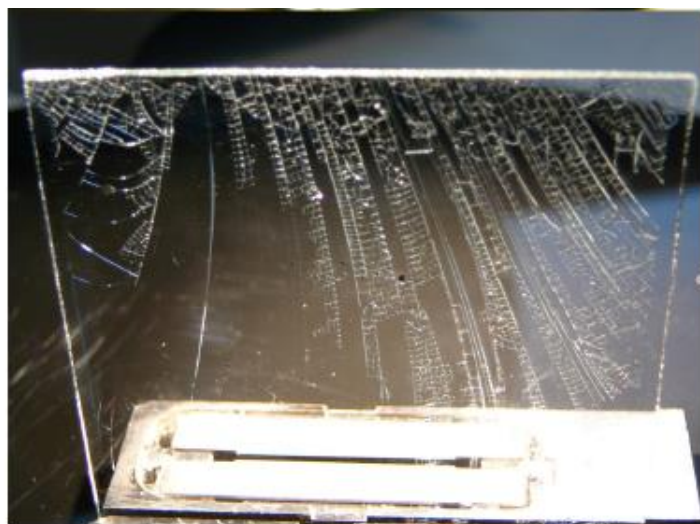
FIG. 7. (Color online) Photographs of the soda lime glass substrate after ALD lithium silicate film deposition at 300 °C.
